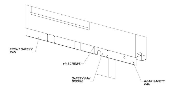
There are eight (8) normally closed (NC) switches that monitor when the safety pan has struck an obstruction. When functioning properly, the switches are actuated only when the safety pan has run into an obstruction, which stops all motion of the platform. The single exception to this is when the platform is within approximately 1/2 inch [13 mm] of the ground, in which case the switches are turned off so that the platform can fully descend to the ground.
