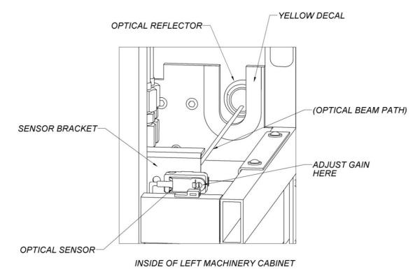
The optical beam must always pass through the area marked with the yellow decal, shown in the figure above. The following procedure can be used if the optical sensor is misaligned:
