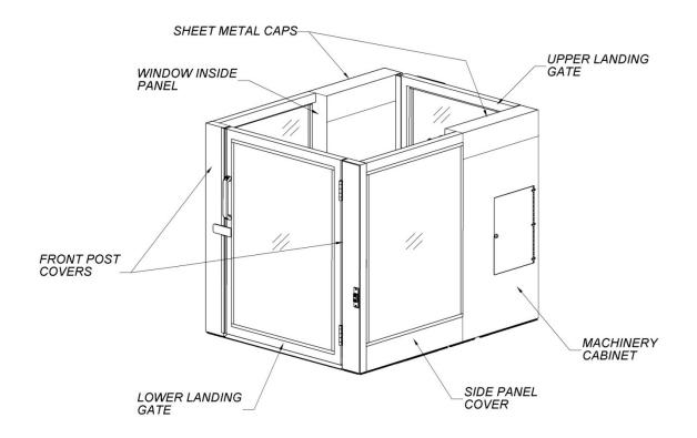
All of the skins are attached to the frame with screws that can be removed with a Phillips screwdriver. Additionally, it may be necessary to remove the grab bar or a window first before removing some of the skins. To remove the grab bar, remove the Phillips head screws that secure it to the lift. To remove a window, refer to Section 3.12.
