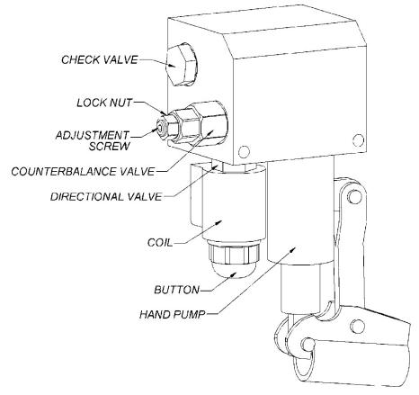
HYDRAULIC MANIFOLD WITH VALVES
