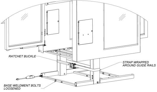
FLOOR, CROSS-MEMBER WELDMENTS, AND SAFETY PAN ASSEMBLY REMOVED
