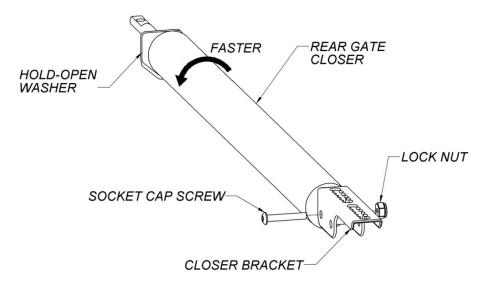
The chain closer is located inside of the bottom of the rear gate. The chain passes between the gate and the frame, with one link of the chain closer held in the chain closer bracket as shown in the figure below.
