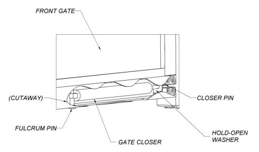
The closer must be removed from inside the gate in order to perform any adjustments. The following procedure can be used to remove and adjust the gate closer:
