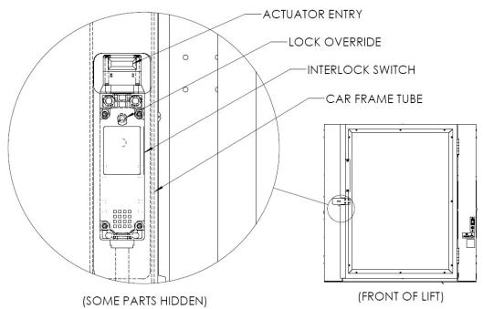
The interlock switch includes a safety circuit that closes only when the gate is closed and locked, as well as a secondary circuit that closes when the gate is closed (regardless of the state of the lock contacts). The locking pin inside the switch is engaged by a spring, and unlocks when the solenoid is energized. The interlock actuator may be inserted even when the solenoid is de-energized.
