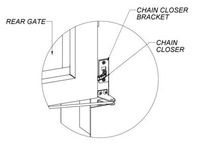
It is not recommended to adjust the chain closer. To remove the chain closer, perform the following procedure:
